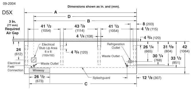
NOTE: Case-to-Case Electrical Connections are made IN FRONT OF SPLASHGUARD.
