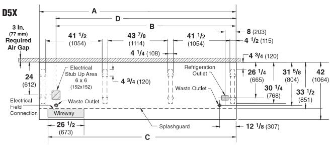
NOTE: Case-to-Case Electrical Connections are made IN FRONT OF SPLASHGUARD.
