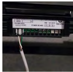
Display is mounted on left side of access panel. Be careful not to detach cable from display when removing access panel.
