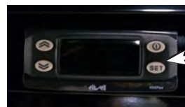
Display is mounted on left side of access panel. Be careful not to detach cable from display when removing access panel.
