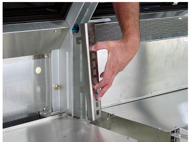
STEP 10 – Lift out lower shelf supports.
