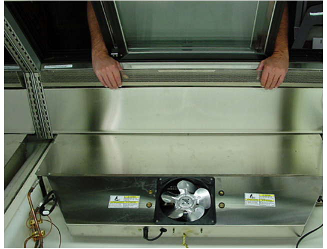
STEP 9 – Lift out upper shelf supports.
