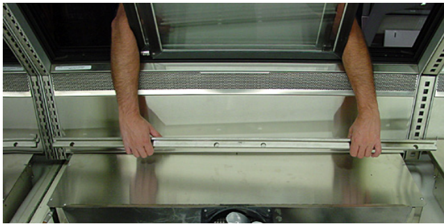
STEP 6 – Lift out display pan support.
