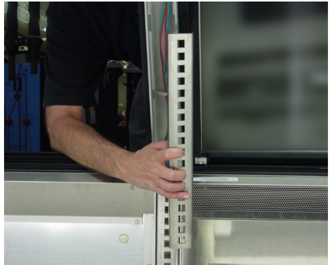
STEP 9 – Lift out upper shelf supports.
