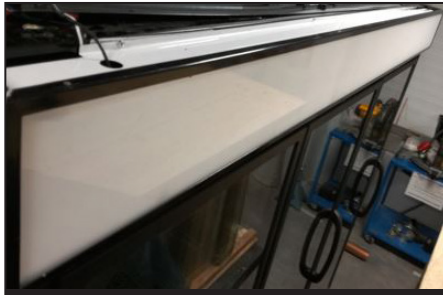
Display Slides out to access Wireway
