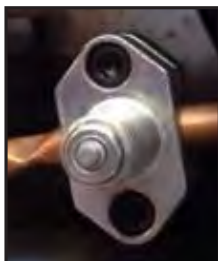
refrigeration line tapping valve
