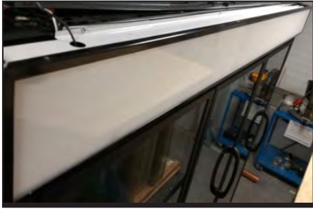
Display Slides out to access Wireway
