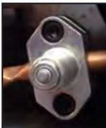
refrigeration line tapping valve
