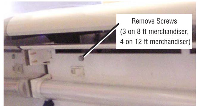
Remove Front Lamp Assembly to Access Screws
