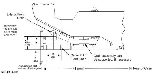
DRAIN EXTENSION KIT REQUIRED TO PIPE MULTIPLE CASES TO ONE DRAIN OR TO USE A RAISED HUB DRAIN
