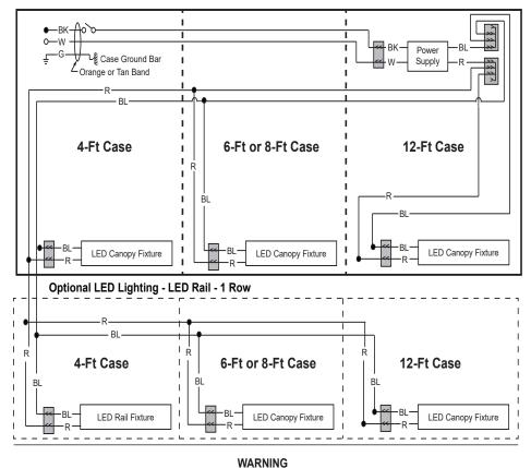
All components must have mechanical ground, and the merchandiser must be grounded.
