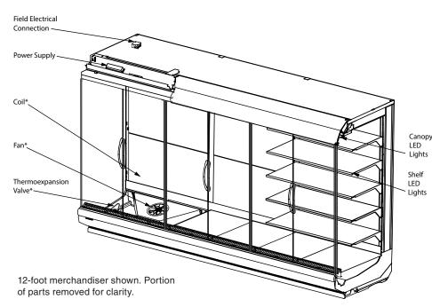
\*Coils, fans, and TXVs are modular with one per 3 or 4-foot section.
