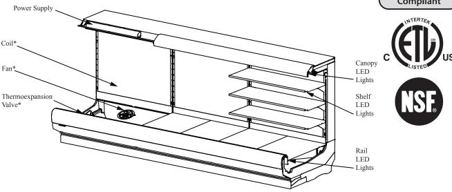
\*Coils, fans and TXVs are modular with one per 3 or 4 foot section.
