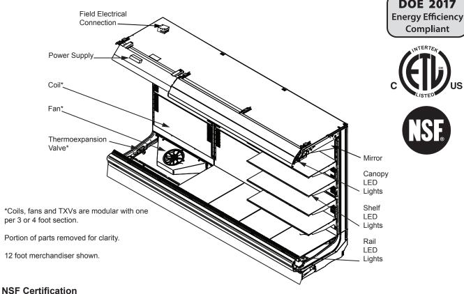
This merchandiser model is manufactured to meet NSF/ANSI (National Sanitation Foundation) Standard #7 requirements for construction, materials and cleanability.
