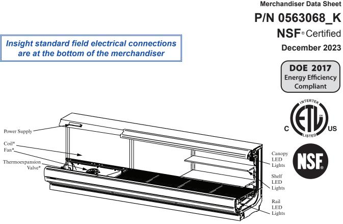
\*Coils, fans and TXVs are modular with one per 3 or 4 foot section.
