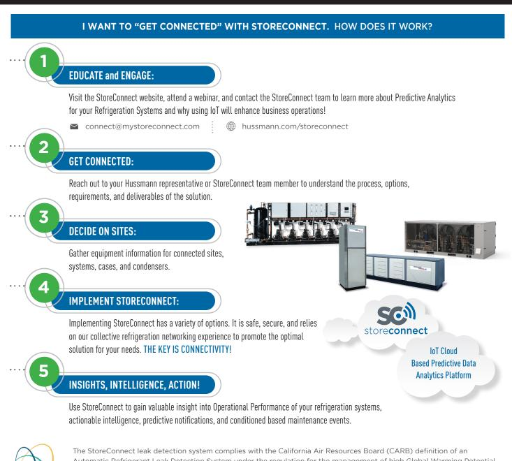
Automatic Refrigerant Leak Detection System under the regulation for the management of high Global Warming Potential (GWP) refrigerants for stationary sources. The CARB regulation states mandatory leak inspections every 90 days on medium size charge systems can be waived if an automatic leak detection system is present.
