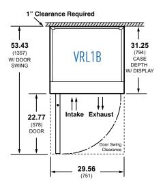
Dimensions are shown as in. and (mm) A clearance of 36 inches is needed in front of the case to ensure no obstruction in the condensing unit air flow. 1 inch clearance required at the top and rear of the case. Zero clearance is required on the sides of the case.
