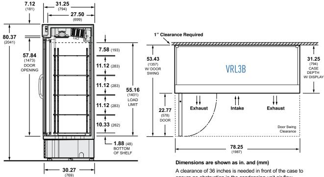
A clearance of 36 inches is needed in front of the case to ensure no obstruction in the condensing unit air flow. 1 inch clearance required at the top and rear of the case. Zero clearance is required on the sides of the case.
