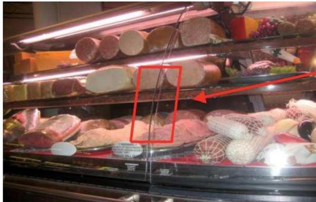
To properly adjust the glass gaps requires that both hinge arms of each section of glass be loosened before attempting to change the glass position.
