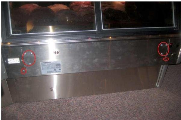
Some cases have wrapping boards installed, the wrapping boards need to be removed to be able to remove the small rear covers. Unhook at K-99 bracket.
