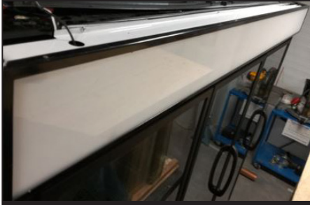
Display Slides out to access Wireway
