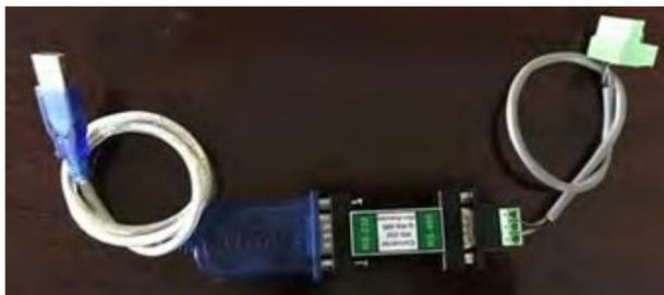
**FIGURA 7: CONVERTIDOR SERIAL**
