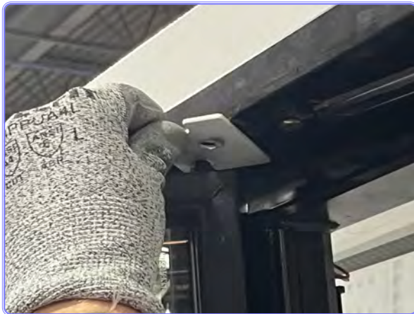
Remove door retaining plate.
