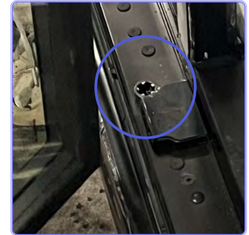
Locate door onto torsion plate hole.
