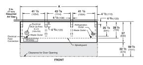
Note: Case-to-case electrical connections are made in front of splashguard. Overall case length without ends or partitions.
