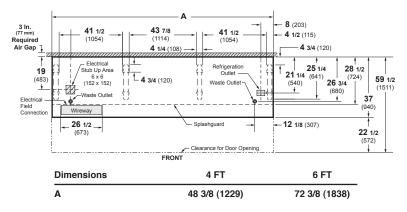
Note: Case-to-case electrical connections are made in front of splashguard. Overall case length without ends or partitions.
