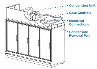
Freedom cases can also be remotely piped to refrigeration racks or condensing units.
