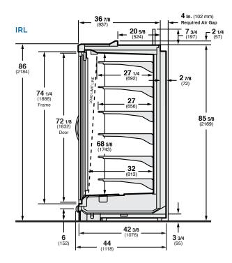
NOTE: These merchandisers are designed for use in stores when temperature and humidity do not exceed 75°F and 55% R.H.
