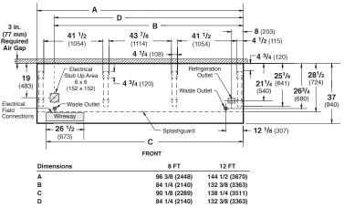
NOTE: Case-to-Case Electrical Connections are made IN FRONT OF SPLASHGUARD.
