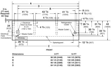
NOTE: Case-to-Case Electrical Connections are made IN FRONT OF SPLASHGUARD.
