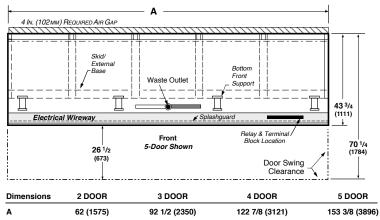
Note: Overall case length without ends or partitions. Each standard end and each insulated partition adds 2 3/4 in. (70mm) to case line up.
