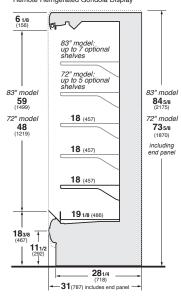
RGD 24, 30 Remote and Self Contained plan view
