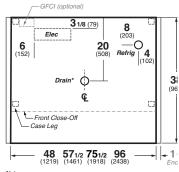
\*Drain position is for 48" length only, refer to Cadblock drawings for other length DOE 2017 Energy Efficiency
