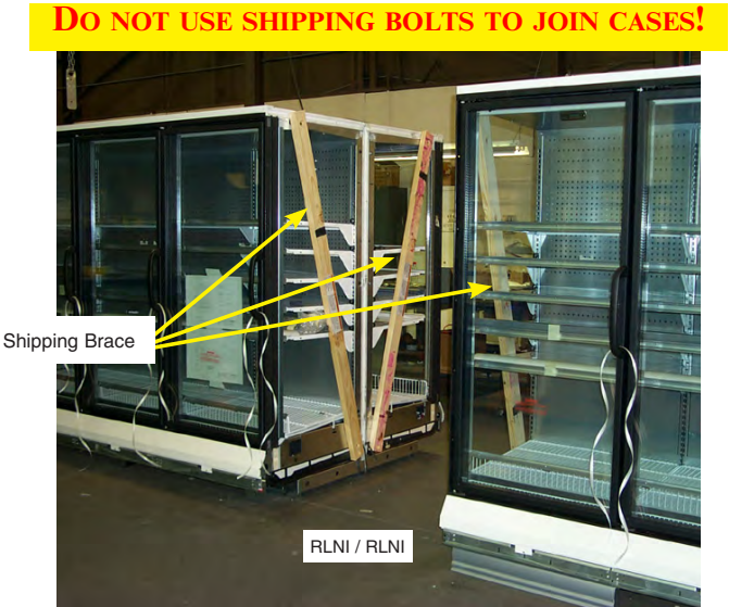
Figure 3. Remove Shipping Braces
