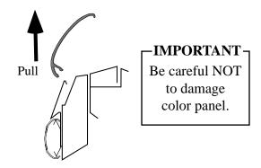
**c.** Remove upper and lower bumpers by pulling bumper away from bumper retainers. Be careful not to lose the internal joint trims on the upper bumpers.
