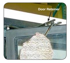
Figure 6. Removing the Door Retainer
