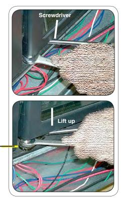
Figure 3. Loosening Torque on the Door
