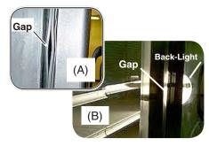
Figure 12. Back-Lighting Gaps in Gasket
