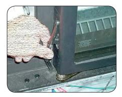
Figure 5. Removing the Heater Terminal Plug
