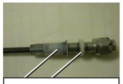
Sleeve bearing and spacer are in excellent condition.
