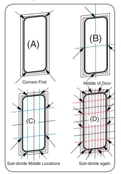
Figure 10. Sequence for Installing New Gasket
