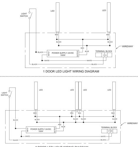
2 DOOR LED LIGHT WIRING DIAGRAM
