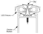
Light Fixture Properly Installed in Clip
