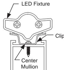
Installing Center Light Fixture into Clip
