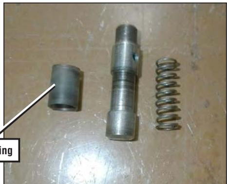
Below is a 5-year-old torque rod that does NOT require maintenance. All components are intact and performing properly.
