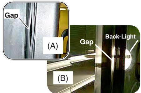
**Figure 12. Back-Lighting Gaps in Gasket**
