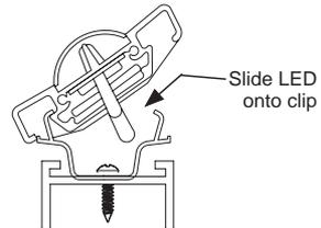
Installing Center Light Fixture into Clip
