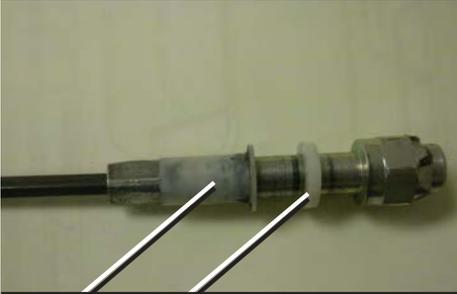
**Sleeve bearing and spacer are in excellent condition.**
