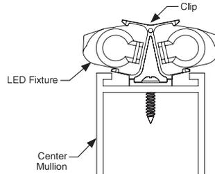
Light Fixture Properly Installed in Clip
