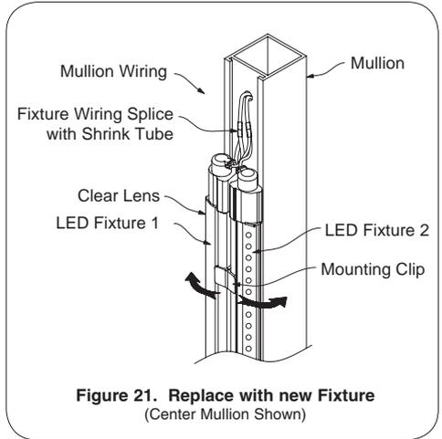
**Figure 21. Replace with new Fixture**
