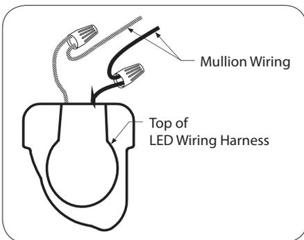
Figure 20. Disconnect Wiring (End Fixture Shown)
