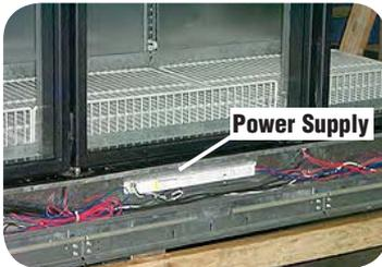
**Figure 22. Power Supply Location**
