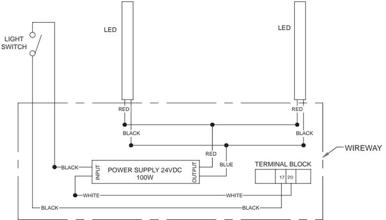
1 DOOR LED LIGHT WIRING DIAGRAM
