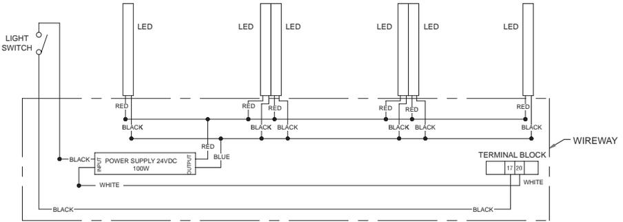
3 DOOR LED LIGHT WIRING DIAGRAM
