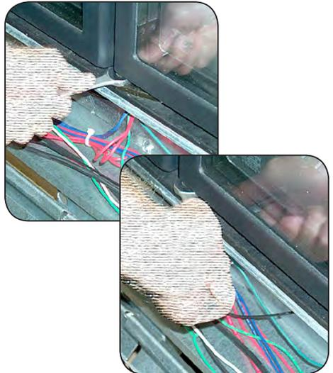
**Figure 1. Adjusting Closing Torque**
