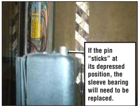
Below is an example of a damaged sleeve bearing. The compromised torque rod components caused the door to "seat" below its designed parameter. Because the door has essentially been lowered, it causes the sleeve bearing to deform. In scenario above, we recommend replacing the torque rod assembly; however, the hinge pin sleeve bearing is a replaceable component.
