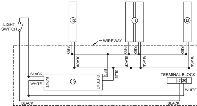
2 DOOR END COMPARTMENT LED LIGHT WIRING DIAGRAM
