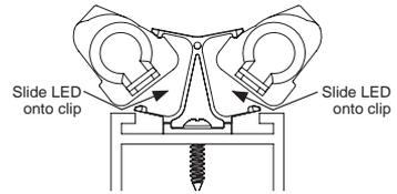
Installing Center Light Fixture into Clip
