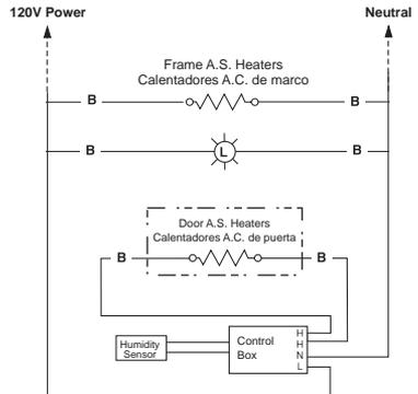
**Wiring Diagram for Controller**
