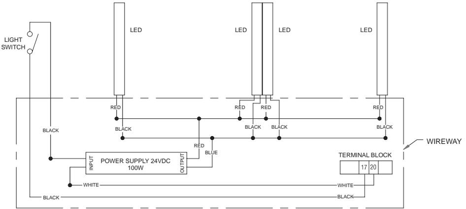
2 DOOR LED LIGHT WIRING DIAGRAM
