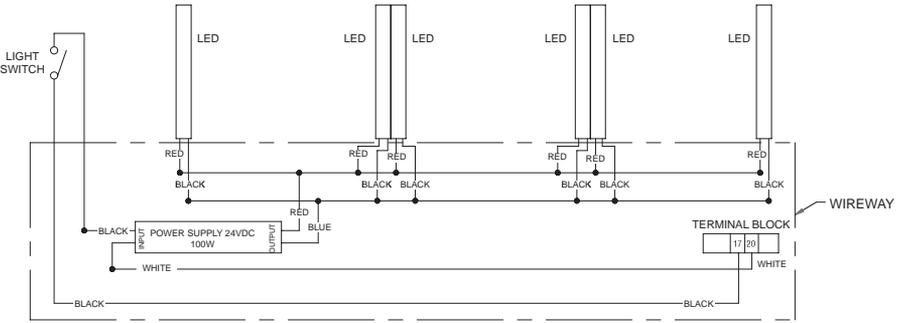
3 DOOR LED LIGHT WIRING DIAGRAM
