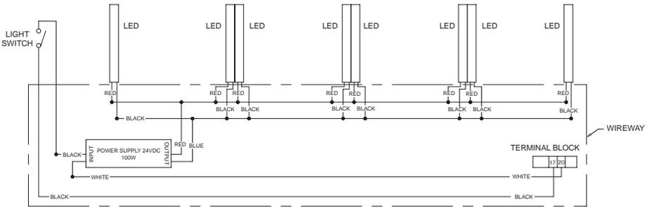
4 DOOR LED LIGHT WIRING DIAGRAM
