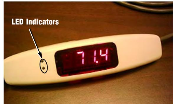
Figure 1. Safe-NET Display Module with Top Cover
