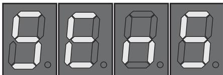
**Alarm with Sensor reading – “noSn”**
