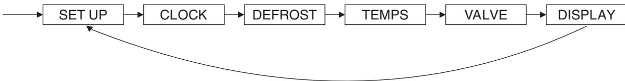
If the unit reverts to the default display due to either an inactivity time-out or use of the escape button sequence, pressing the SELECT button will advance to the next top-level menu in sequence as shown above.
