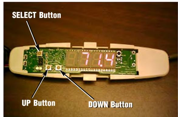
Figure 2. Safe-NET Display Module with Cover Removed
