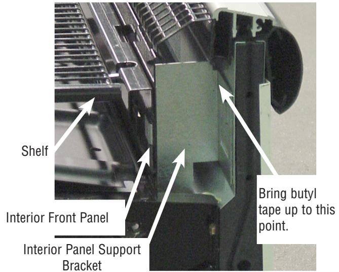
2. Apply butyl tape across the bottom joint. Be sure to extend the tape up the back and front of the merchandiser.
