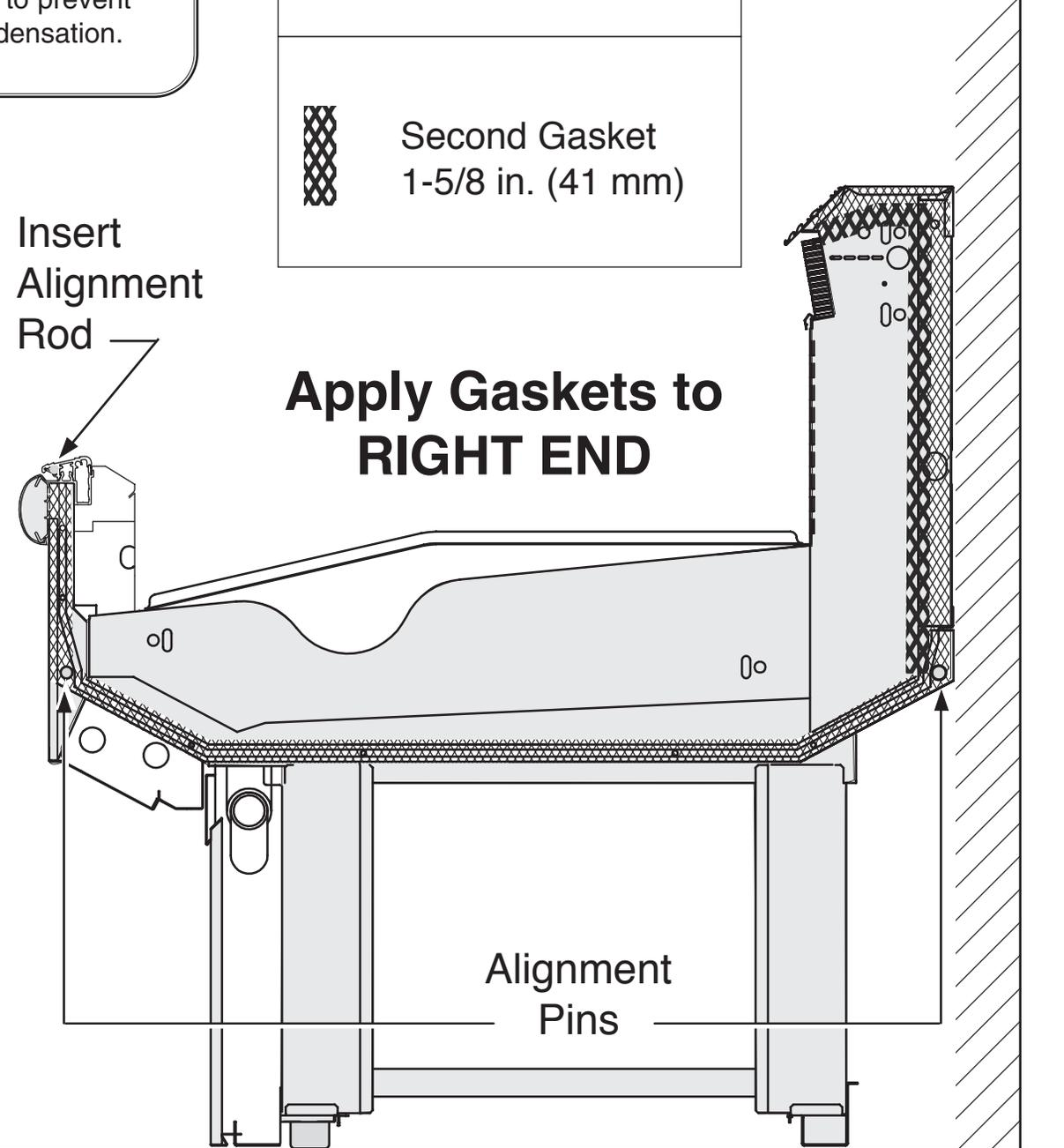
**Gasket Location for Joining (Single Deck)**
