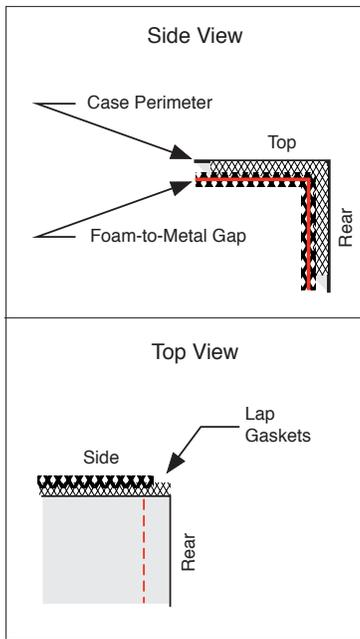
**Gasket Location for Joining (Multi-deck)**
