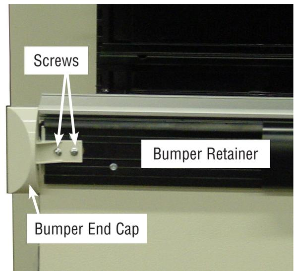
4. Starting at the left end of the lineup, install the bumper starter section first. To install:
