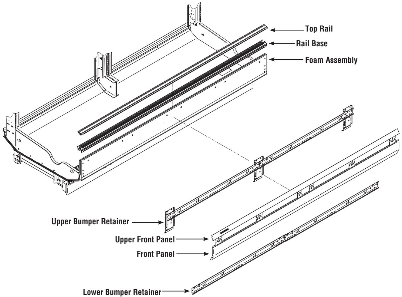
6. Verify that each merchandiser's upper front panel, front panel, and top rail align before joining merchandisers. Panels and top rail must have equal overhang at each end of the merchandiser.
