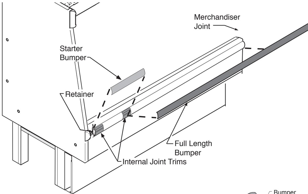
b. Install full-length bumpers and internal trims offset across joints. Make sure that no gaps exist between sections. Continue installing the bumpers the length of the lineup.
