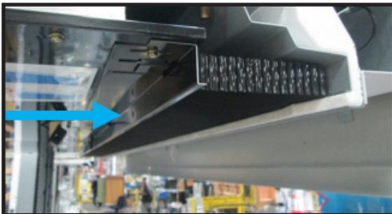
2. Loosen or remove screws that hold retainer in place.
