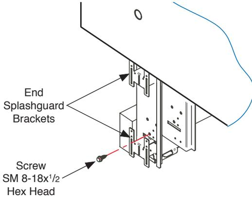
b. Align forward edge of End Splashguard with front splashguard, with lower edge resting on floor. Fasten End Splashguard to bracket with Screws.
