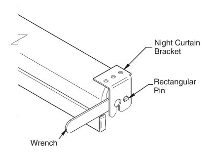
Put the Spindle Lock (parts list Item 4) on the round spindle of the night curtain. The spindle is on the left end of the night curtain. Put the spindle lock in place by sliding it into the keyhole slot of the left bracket and turning the spindle lock 90 degrees as shown in the illustration.
