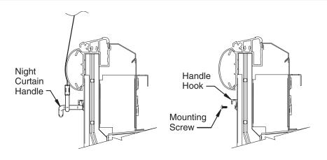
Mount the Handle Hook (parts list Item 5) below the front bumper. Pull the night curtain down and put the hook on the handle to position the hook.
