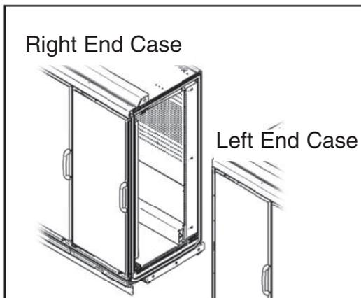
**Use all three gaskets when applying an end assembly.**
