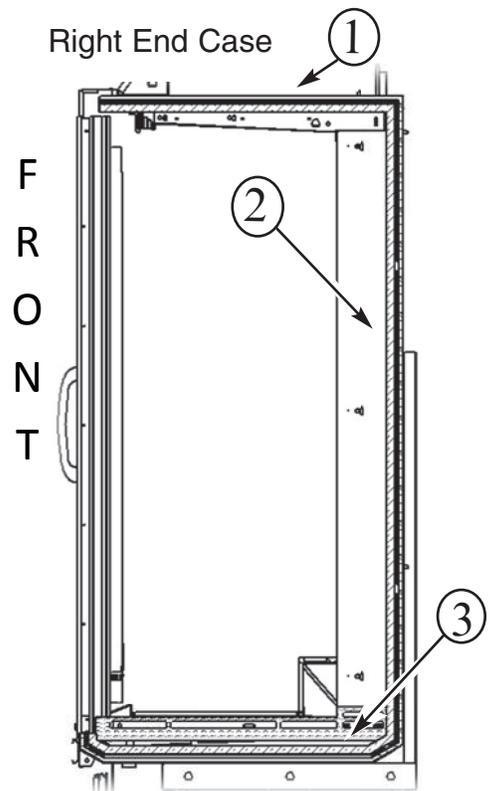
**Use only one right Gasket Pad Sealer for each case joining.**
