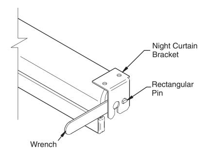
Put the **Spindle Lock** (parts list **Item 4**) on the round spindle of the night curtain. The spindle is on the left end of the night curtain. Put the spindle lock in place by sliding it into the keyhole slot of the left bracket and turning the spindle lock 90 degrees as shown in the illustration.
