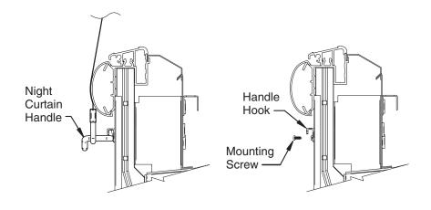
Once the Night Curtain installation is complete, spring tension cannot be adjusted without removing the curtain from the case.
