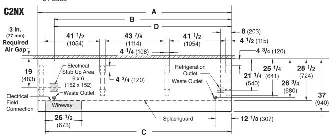
NOTE: Case-to-Case Electrical Connections are made IN FRONT OF SPLASHGUARD.
