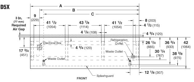
Note: ALL FIELD WIRING CONNECTION POINTS ARE ABOVE THE CASE. Case to case connections are made in the electrical box at the top of the case.
