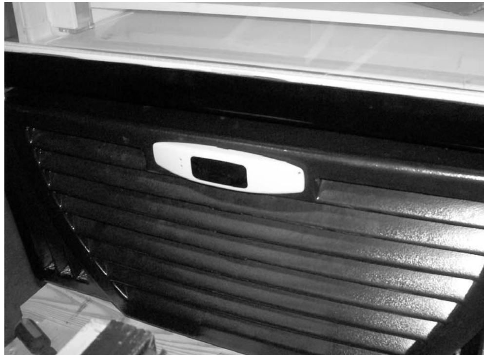
The Safe-NET electronic controller is located on the front of the lower front grille.
