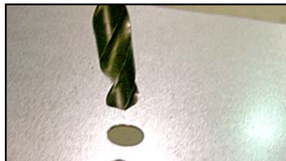
Drill \frac{1}{4} in. Hole(s) in Light Channel
