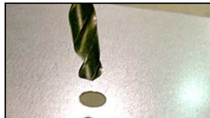
Drill \frac{1}{4} in. Hole(s) in Light Channel
