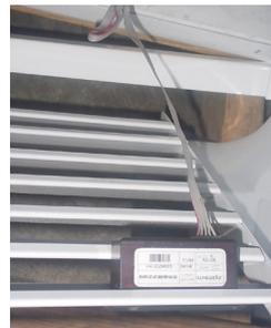
Safe-NET III display is mounted on left side of access panel. Be careful not to detach Safe-NET III cable from display when removing access panel.
