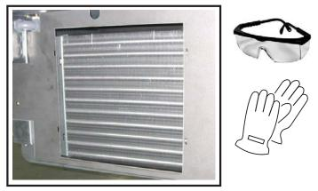
Airflow blockage increases energy consumption and reduces the merchandiser's ability to maintain operating temperature.
