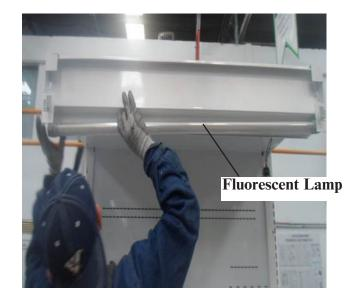
3. The ballast is located under the top sign.
