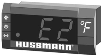
If the merchandiser sensor fails, refrigeration will run continuously. Turn off, or repeat a duty cycle of a few minutes on and a few minutes off.
