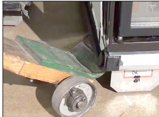
**Use J-Bar to Align Cases for Joining**
