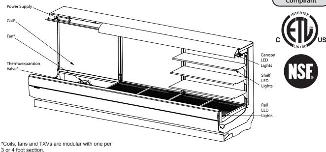
Portion of parts removed for clarity.
