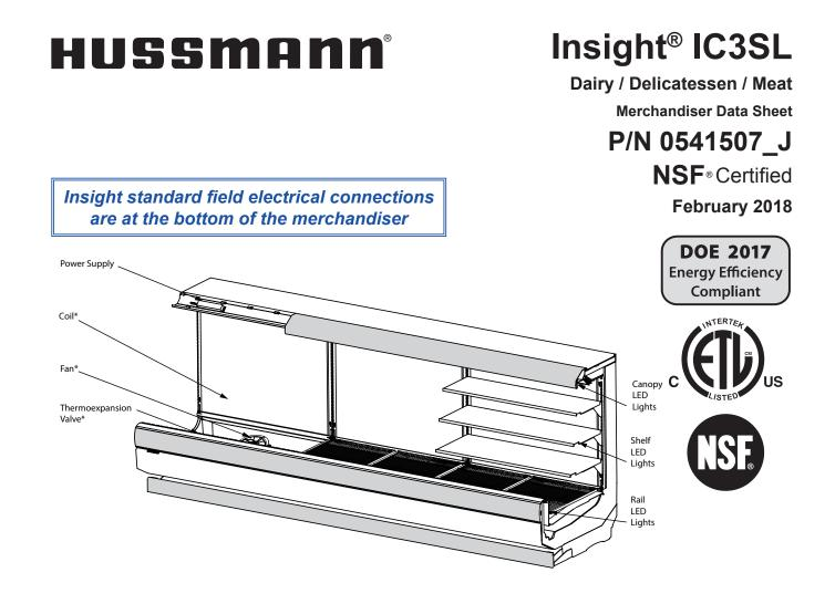
\*Coils, fans and TXVs are modular with one per 3 or 4 foot section.
