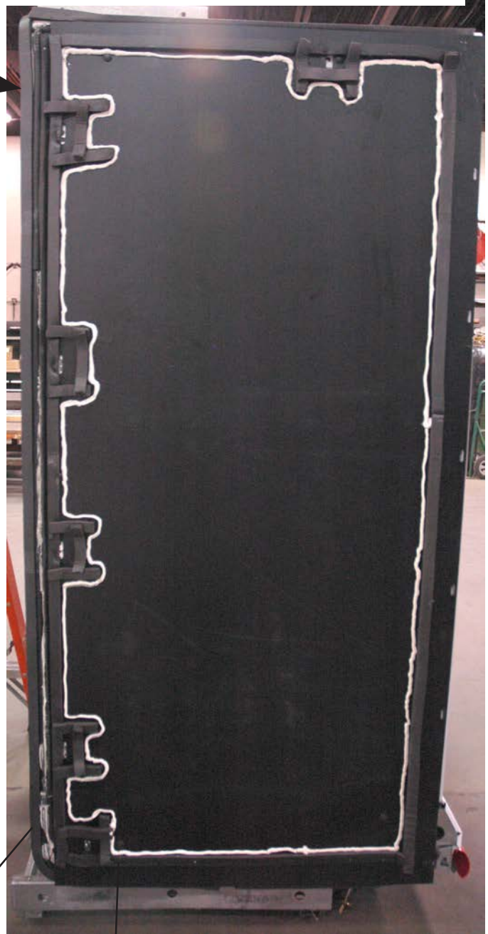
Figure 4: Apply Butyl Sealer
